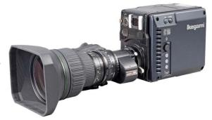
camera with the purchase of a software license. Employing the same sensors as the UHK-430/435 "UNICAM XE" series cameras, the UHL-43 produces superb high quality images. In addition, due to its compact one-piece form factor, it is suitable for pan-tilt camera systems and monitoring cameras that shoot their subjects from various angles.
